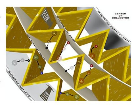
system, while one with an inherent negative charge is drawn toward a grounded plate. A charge-neutral particle that either is already highly polar in nature, or is polarized by the non-uniform voltage field of the collector is drawn toward the area of the greatest field strength (folds of the collector pleats).
